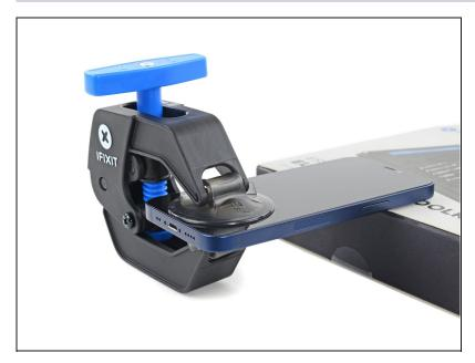
Place a support under your device so the Anti-Clamp stands upright without being held in place.
