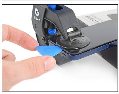
Insert an opening pick into the gap created by the Anti-Clamp.
