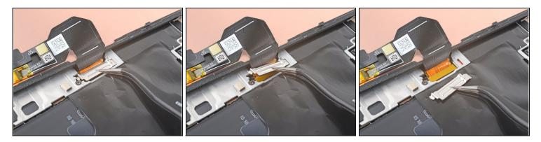
(i) The display cable bracket is secured with metal clips.
