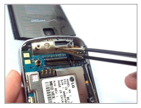
With a pair of tweezers, pull the gold flex cable up disconnecting the motherboard.
