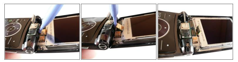
• Use the plastic opening tool to gently pry the LCD cable out of its socket.
