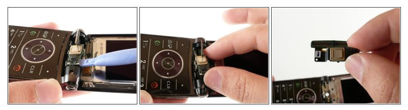
• Use a plastic opening tool to gently pry the camera assembly away from the RAZR2.
