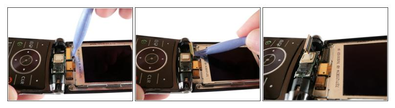
• Use the plastic opening tool to gently pry the motherboard cable out of its socket.
