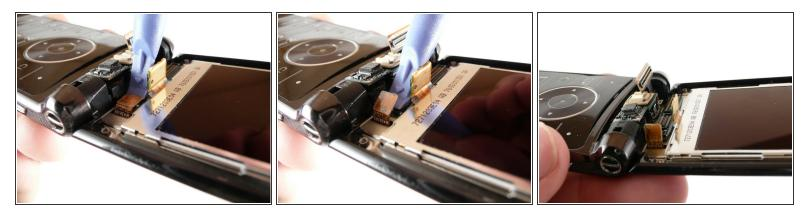
• Use the plastic opening tool to gently pry the camera cable out of its socket.
