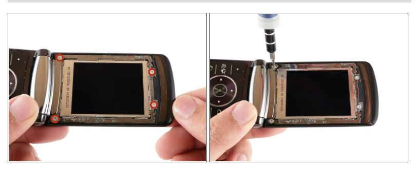
Remove the four 2-mm T5 Torx screws
