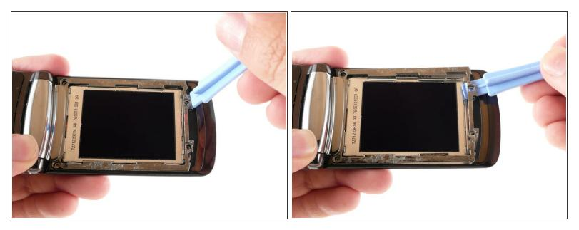
• Use a plastic opening tool to pry the top end of the metal frame away from the RAZR2.
