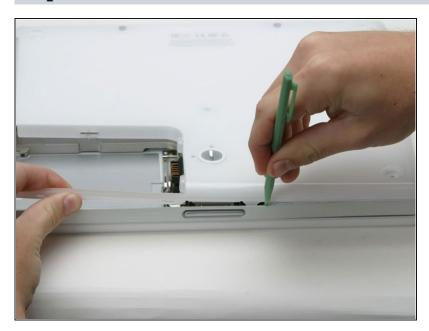
PRUN a spudger along the seam between the lower case and upper case on the front of the computer to free the tabs locking the lower case. Pull up on the lower case and continue to use the spudger as necessary until you hear three distinct clicks.
