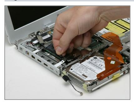
Deroute the display data and microphone cables.
