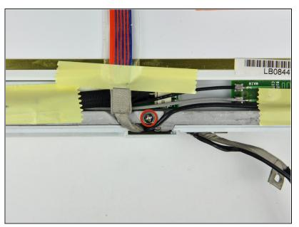
Remove the second of the two Phillips screws securing the clutch cover to the cast aluminum frame of the clutch hinges.
