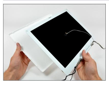
Lift the rear bezel off the display.
