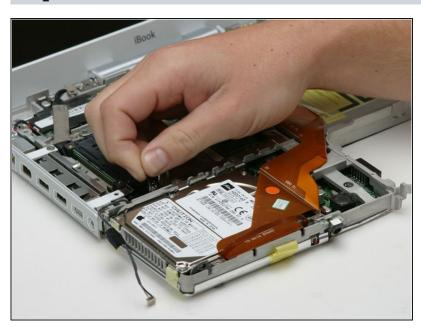
Use the black plastic handle to disconnect the display data cable from the logic board.
