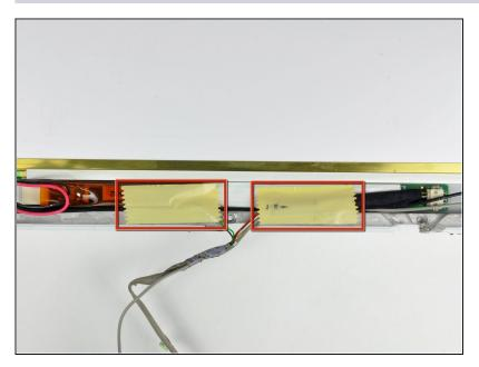
Remove the two pieces of tape covering the inverter/AirPort cables along the lower edge of the display.
