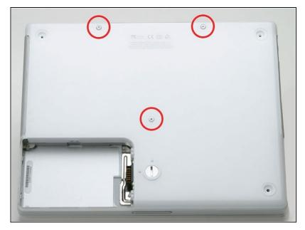
Remove the one 10 mm and two 20 mm hex screws using a 2mm hex. Alternatively, a T8 Torx screwdriver key will do.
