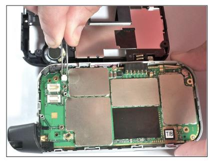
Using tweezers, pull on the connector or wire in the direction of the wire with gentle pressure to unplug the wire connector from the motherboard.
