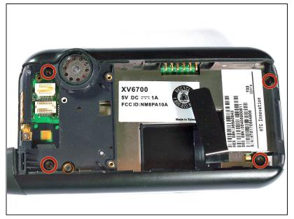
• Remove the four 5.0-mm Torx T6 screws from the corners of the black cover.
