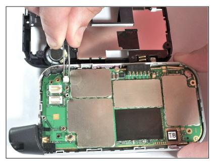
Using tweezers, pull with gentle pressure in the direction of the wire to unplug from the motherboard connector.
