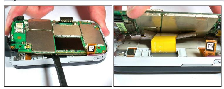
• Carefully lift up on the motherboard with the spudger until you can see the display cable connected to the underside of the motherboard. The display cable connector will be taped over.
