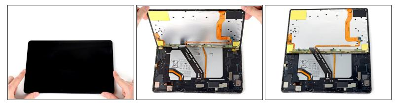
A Don't try to remove the screen all the way yet; it's still connected by a flex cable.
