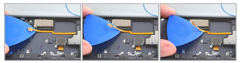
Slice with the opening pick along the bottom of the connector's cable to completely separate it from the frame.
