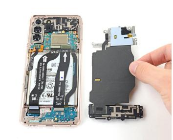
Use a pair of tweezers or your fingers to carefully remove the NFC antenna and charging coil assembly.
