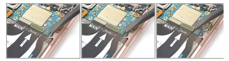
• Use a spudger to pry up and disconnect the primary and secondary interconnect cables' press connectors on the motherboard.
