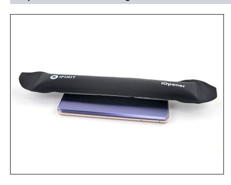
Heat an iOpener and apply it to the left edge of the back cover for two minutes.
