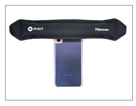
Heat an iOpener and apply it to the top edge of the back cover for two minutes.
