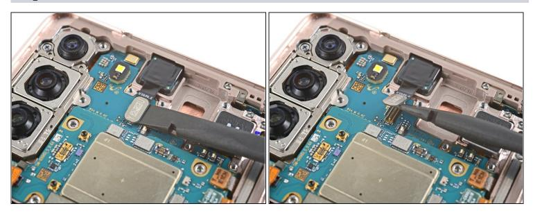
• Use a spudger to pry up and disconnect the front camera's press connector.
