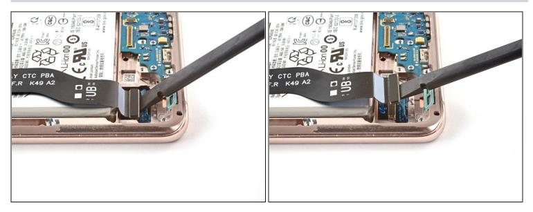
• Use a spudger to pry up and disconnect the display cable's press connector near the bottom of the device.
