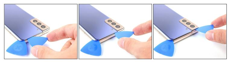
A When you slice near the camera assembly, insert only the tip of the opening pick (~4-5 mm) to avoid damaging or smearing the camera.
