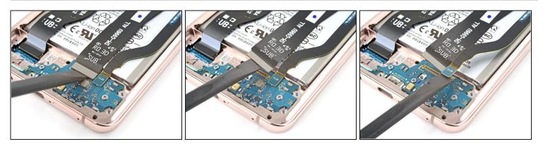
• Use a spudger to pry up and disconnect the primary and secondary interconnect cables' press connectors on the daughterboard.
