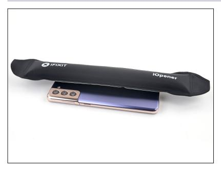
• <u>Heat an iOpener</u> and apply it to the right edge of the back cover for two minutes.
