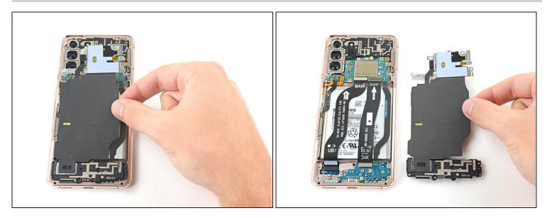
• Use a pair of <u>tweezers</u> or your fingers to carefully remove the NFC antenna and charging coil assembly.
