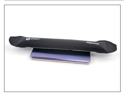
• <u>Heat an iOpener</u> and apply it to the left edge of the back cover for two minutes.
