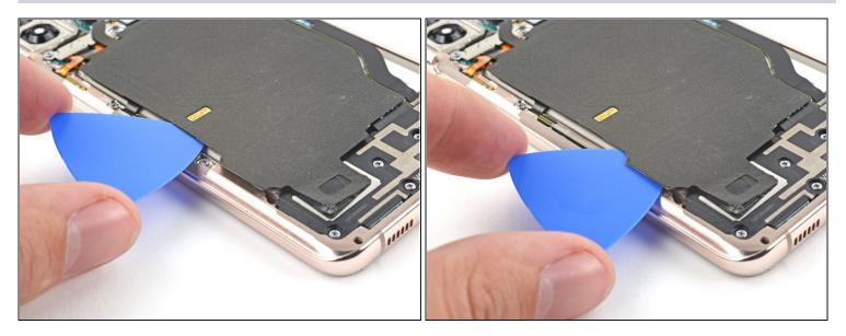
Take care not to puncture or bend the battery with your tool—a punctured or bent battery may leak dangerous chemicals or cause a thermal event.
