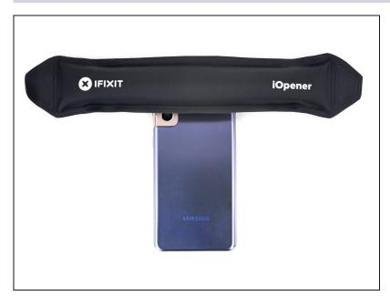
• <u>Heat an iOpener</u> and apply it to the top edge of the back cover for two minutes.
