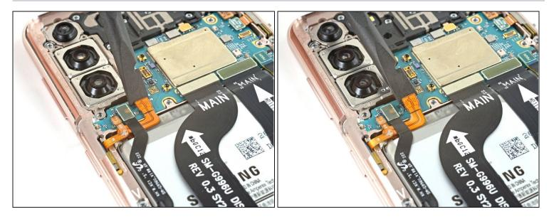
• Use a spudger to pry up and disconnect the battery's press connector.
