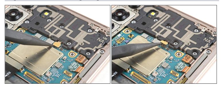
• Use the tip of a spudger to pry up and disconnect the earpiece speaker's press connector.
