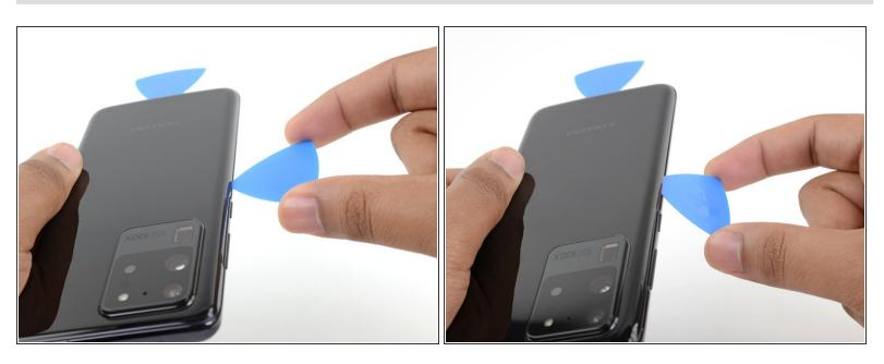
Once the pick is underneath the glass's edge, tilt it downward and insert it further to fully separate the back cover's adhesive.
