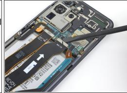
Use a spudger to pry up and disconnect the primary and secondary interconnect cables from the motherboard.
