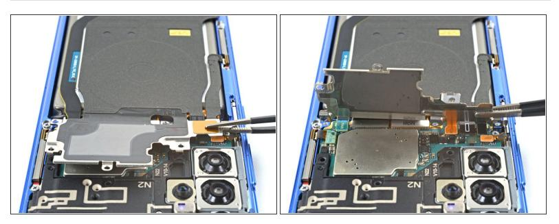
• Gently tilt up the motherboard bracket so the orange battery connector is accessible.
