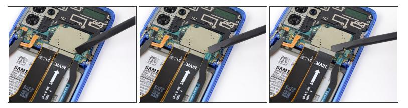
• Use a spudger to pry up and disconnect the primary and secondary flex cables from the motherboard.
