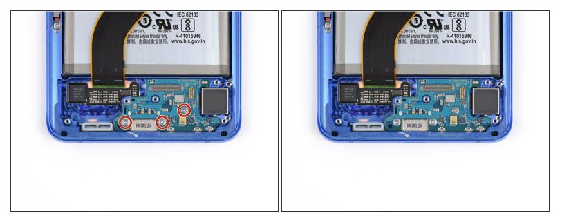
Use a Phillips #00 screwdriver to remove the three 3.4 mm-long screws securing the USB-C port and daughterboard.
