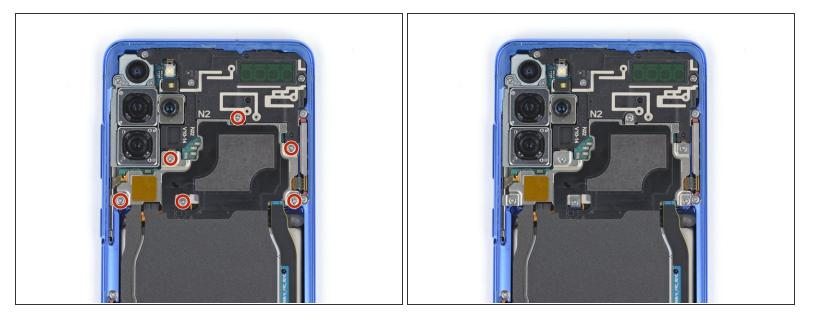
Use a Phillips #00 screwdriver to remove the six 4 mm-long screws securing the motherboard bracket.
