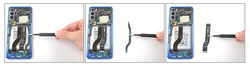
• Gently peel up and remove the primary and secondary flex cables.
