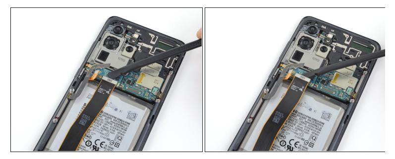
• Pry up and disconnect the display flex cable from the motherboard.
