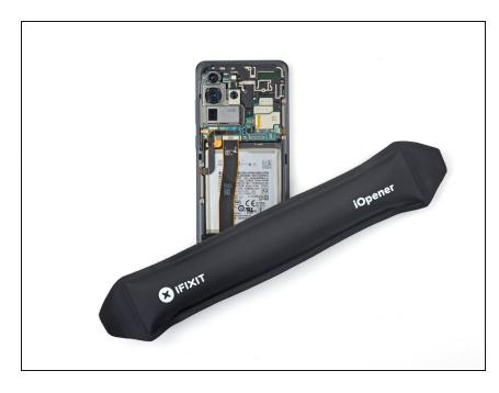
• Apply a heated iOpener to the bottom-right of the device for 90 seconds.
