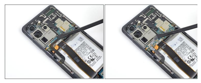
• Pry up and disconnect the left 5G mmWave antenna connector from the motherboard.
