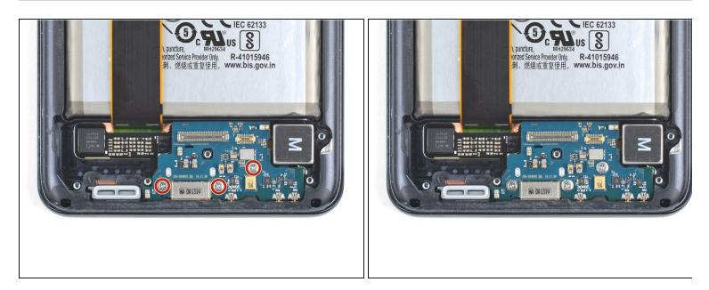
Use a Phillips #00 screwdriver to remove the three 3.7 mm-long screws securing the USB-C port and daughterboard.
