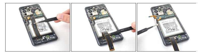
• Gently peel up and bend the display and left 5G mmWave antenna flex cables out of the way of the motherboard and battery.
