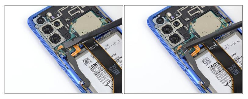
Pry up and disconnect the left 5G mmWave antenna cable from the motherboard.
