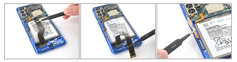
• Gently peel up and bend the display and left 5G mmWave antenna flex cables out of the way of the motherboard and battery.
