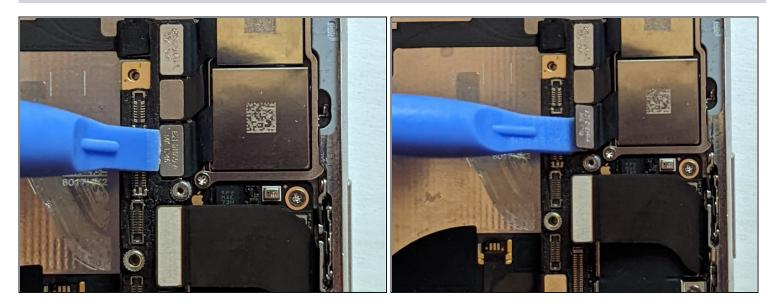
• Disconnect the Telephoto Camera cable connector.
