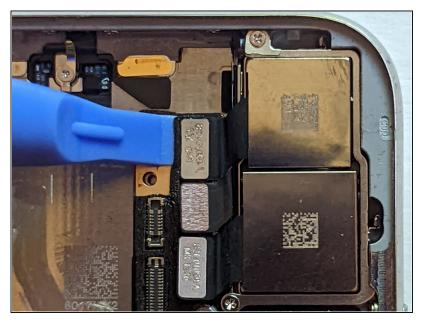
• Disconnect the Wide-Angle Camera cable connector.
