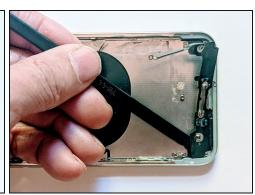
• Peel off the cable with a spudger.
