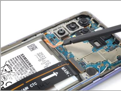
• Use a spudger to disconnect the battery cable by prying the connector straight up from its socket.
