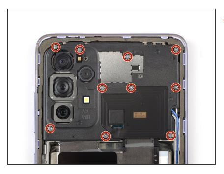
Use a Phillips screwdriver to remove the ten 4.5 mm-long screws securing the motherboard cover.
