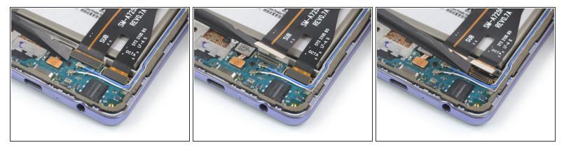
Use a spudger to disconnect both ends of the interconnect cable by prying the connectors straight up from their sockets.
