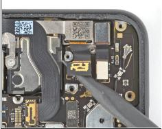
• Use the pointed end of your spudger to pry the camera and sensor connectors straight up from the motherboard to disconnect them.
