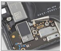
Use a pair of tweezers to disconnect the two coaxial antenna connectors from the motherboard.
