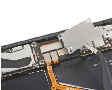
• Use a pair of tweezers to remove the display connector cover.
