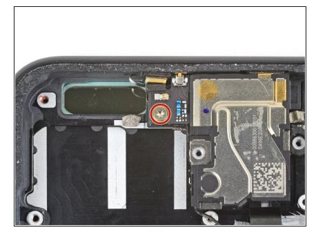
Use a T3 Torx driver to remove the 2 mm screw securing the antenna connector board board to the phone.
