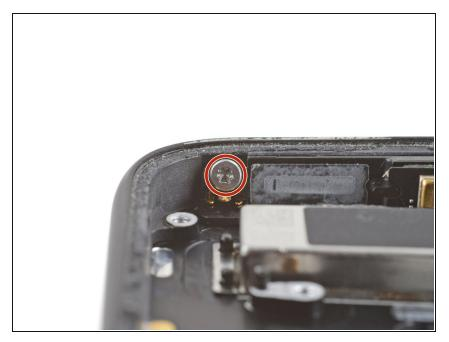
Use a T3 Torx driver to remove the 3 mm screw securing the bottom microphone assembly to the bottom right corner of the frame.
