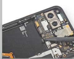
• Use the pointed end of your spudger to disconnect the three side button and rear-facing camera connectors from the motherboard.
