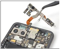
• Use a pair of tweezers to remove the front camera and sensor assembly.
