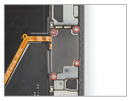
Use your T3 Torx driver to remove the four 3.5 mm screws securing the display connector cover.
