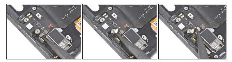
Disconnect the antenna press connectors from the charging assembly.
