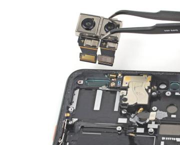
• Use a pair of tweezers to remove the rear-facing camera module.
