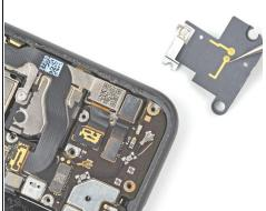
Use a pair of tweezers to remove the front-facing camera connector cover.
