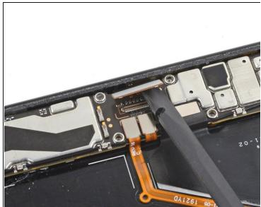
• Use the flat end of a spudger to disconnect the display connector from the motherboard.
