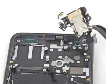
• Use a pair of tweezers to remove the earpiece speaker and Soli motion sensor assembly.
