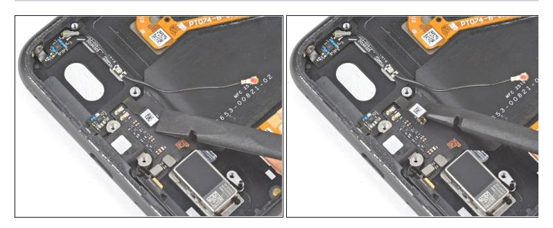
Use the pointed end of your spudger to disconnect the two antenna press connectors from the charging assembly.
