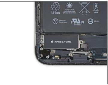
• Remove the two 1.9 mm Phillips screws securing the Taptic Engine.
