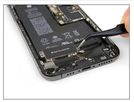
Remove the Taptic Engine assembly.
