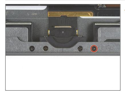
Use a Phillips screwdriver to remove the 2.3 mm-long screw securing the right speaker.
