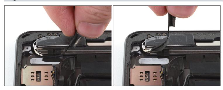
• Continue to peel the right antenna cable away from the rear case.
