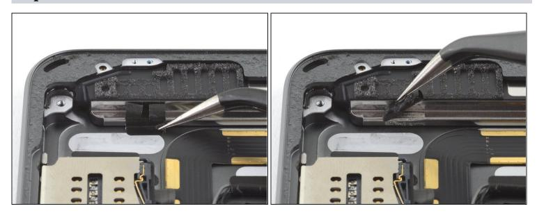
• Carefully peel the LCD buffer tape away from of the rear case.
