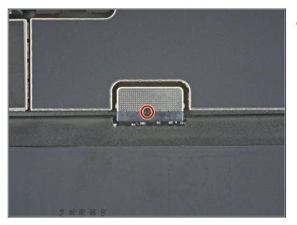
Use a Phillips screwdriver to remove the single 2.3 mm-long screw securing the battery connector to the logic board.
