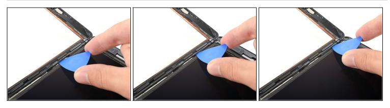
• While supporting the digitizer, slide an opening pick between the two display cables to separate the last of the adhesive.
