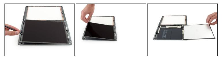
⚠ Don't attempt to fully remove the LCD during this step, as it's still connected by several cables at the home button end.
