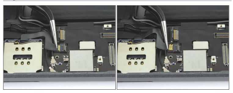
• Use a pair of tweezers to carefully pull the SIM card reader cable straight out of the ZIF connector.
