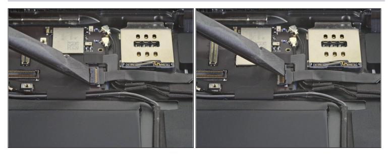
• Use the tip of a spudger, an opening tool, or your fingernail to flip up the small, hinged locking flap on the home button cable <u>ZIF connector</u>.
