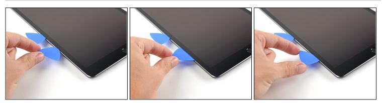
• If the opening pick gets stuck in the adhesive, "roll" the pick along the side of the iPad to continue separating the adhesive.
