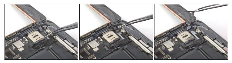
Use a pair of tweezers to peel the home button cable away from the rear case.
