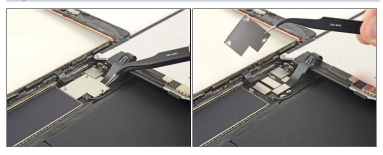
• Remove the display cable bracket.
