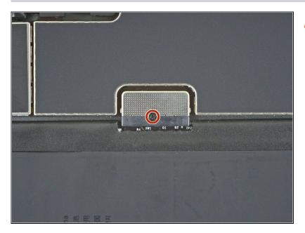
• Use a Phillips screwdriver to remove the single 2.3 mm-long screw securing the battery connector to the logic board.
