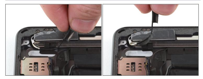
• Continue to peel the right antenna cable away from the rear case.
