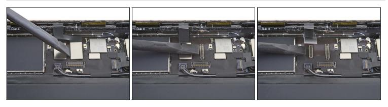
• Use the flat end of a spudger to disconnect the two digitizer cables by lifting straight up on the press connectors.
