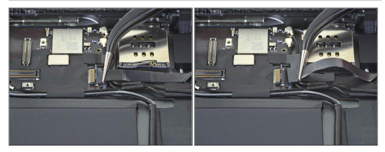
• Use a pair of tweezers to carefully pull the home button ribbon cable straight out of the ZIF connector.
