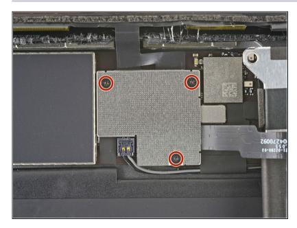
• Use a Phillips screwdriver to remove the three 1.4 mm-long screws securing the display cable bracket.
