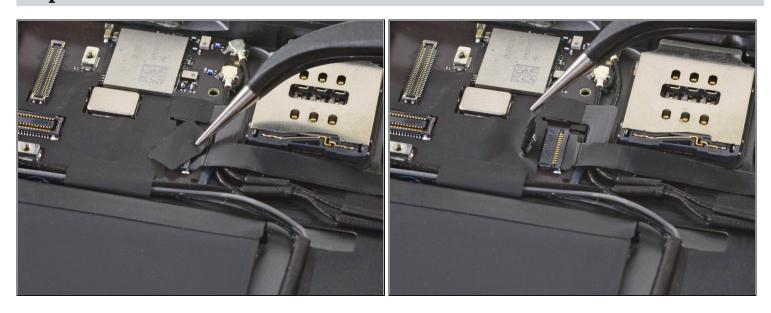
Use a pair of tweezers to peel off the tape covering the home button cable ZIF connector.
