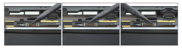
• Use the tip of a spudger, an opening tool, or your fingernail to flip up the small, hinged locking flap on both the left and right speaker cable ZIF connectors.
