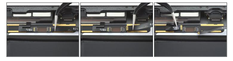
• Use a pair of tweezers to carefully pull the left and right speaker cables straight out of their respective ZIF connectors.
