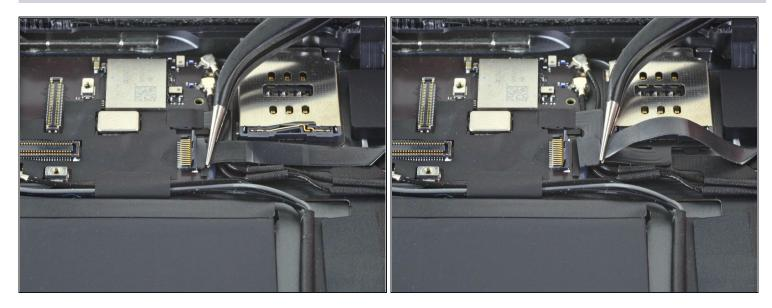
• Use a pair of tweezers to carefully pull the home button ribbon cable straight out of the ZIF connector.
