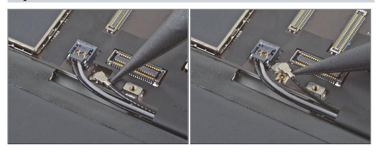
• Use the pointed end of a spudger to disconnect the Smart Connector coaxial cable by prying up as close to the connector as possible.
