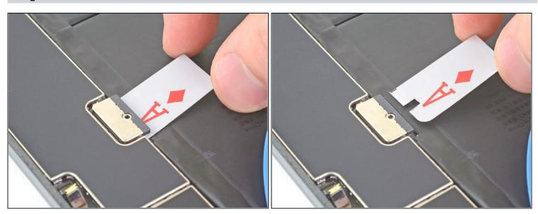
Remove the battery blocker.
