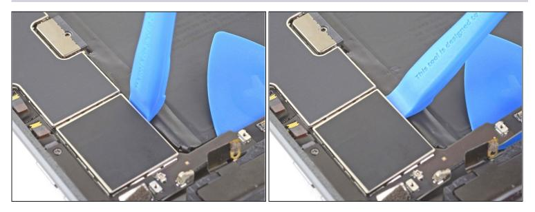
• Insert an opening tool near the top of the logic board and pry up with a slow and steady force to peel it away from the rear case.
