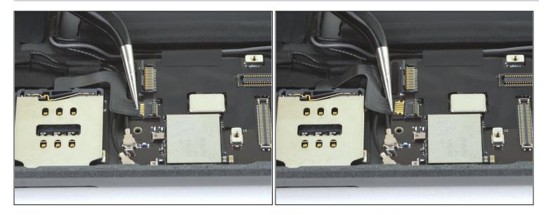
• Use a pair of tweezers to carefully pull the SIM card reader cable straight out of the ZIF connector.
