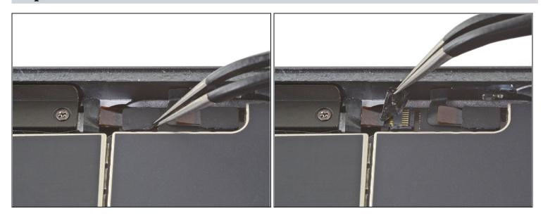
• Peel off any tape covering the <u>button control cable ZIF connector</u>.
