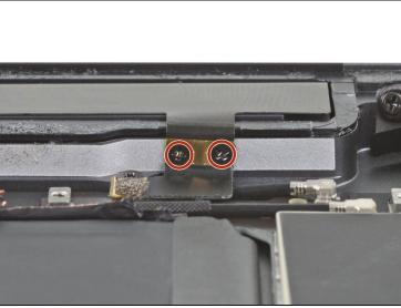
• Use a Phillips screwdriver to remove the three 1.4 mm-long screws securing the cellular antennas to the rear case.
