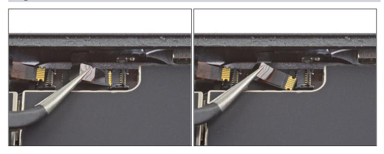
• Use a pair of tweezers to carefully pull the Smart Cover sensor cable straight out of the ZIF connector.
