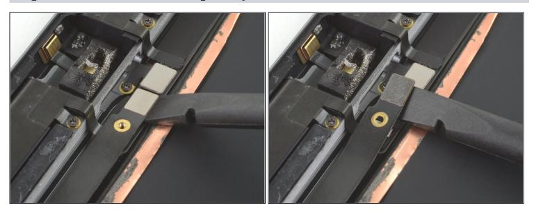
• Use the flat end of a spudger to disconnect the headphone jack by lifting straight up on the press connector.
