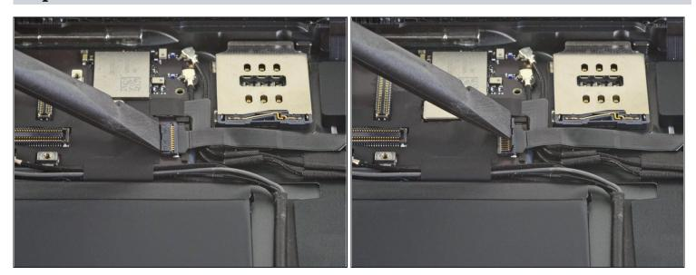
• Use the tip of a spudger, an opening tool, or your fingernail to flip up the small, hinged locking flap on the home button cable <u>ZIF connector</u>.
