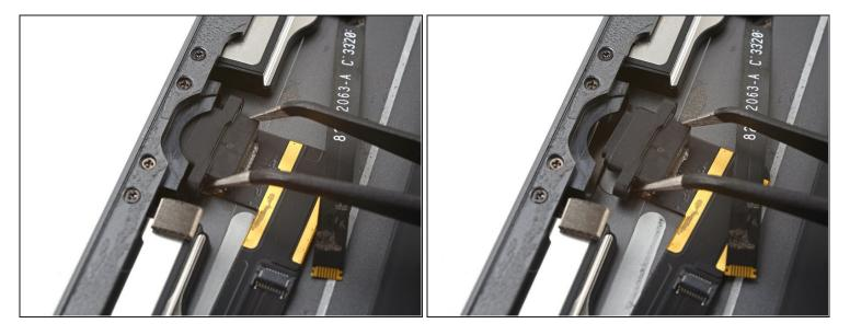
• Pull the charging port out of its slot in the rear case.
