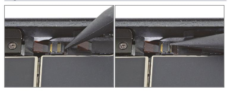
• Use the tip of a spudger, an opening tool, or your fingernail to flip up the small, hinged locking flap on the button control cable ZIF connector.
