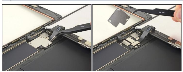
• Remove the display cable bracket.
