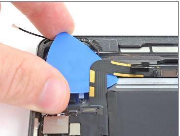
• Insert an opening pick under the charging port cable near the logic board and slide it toward the charging port to slice the adhesive.
