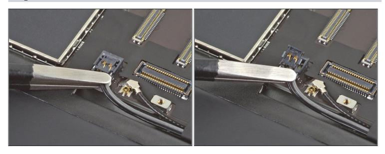
Use a pair of tweezers to disconnect the Smart Connector cable connector by lifting straight up.
