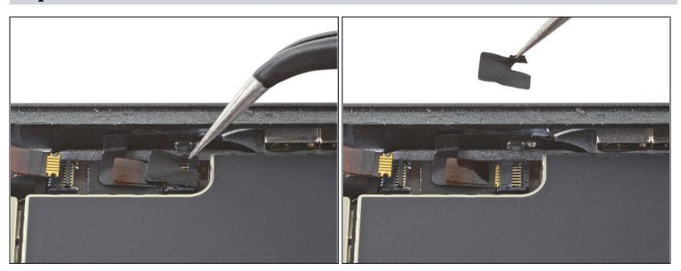
• Peel off any tape covering the Smart Cover sensor cable ZIF connector.
