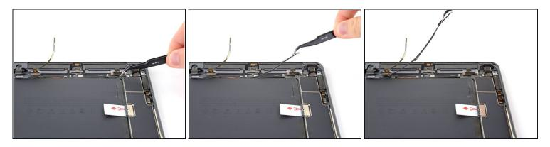
• Peel the left cellular antenna coaxial cable away from the rear case.
