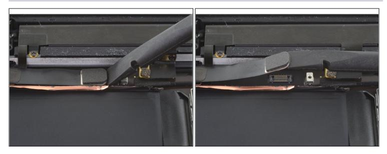
Use the flat end of a spudger to disconnect the front camera cable by lifting straight up on the press connector.
