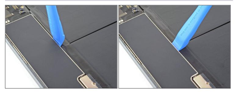
• Insert an opening tool near the middle of the logic board and pry up with a slow and steady force to peel it away from the rear case.
