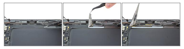
Use a pair of tweezers, or your fingers, to peel up the tape covering the speaker connectors.
