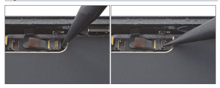
• Use the tip of a spudger, an opening tool, or your fingernail to flip up the small, hinged locking flap on the Smart Cover sensor cable ZIF connector.
