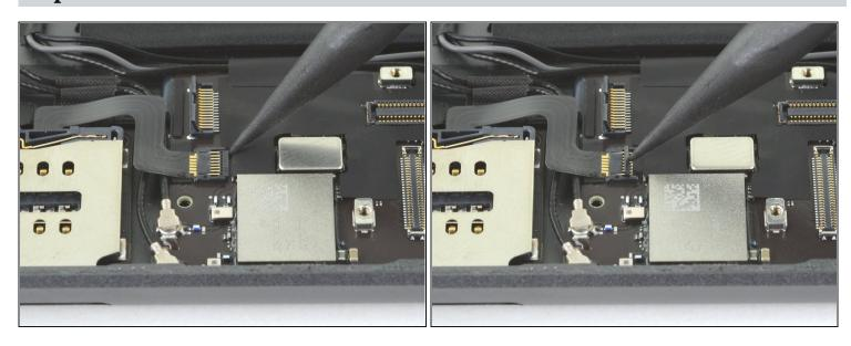
• Use the tip of a spudger, an opening tool, or your fingernail to flip up the small, hinged locking flap on the SIM card reader cable ZIF connector.
