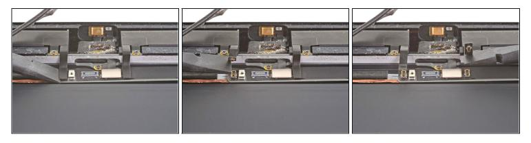
Use the flat end of a spudger to disconnect both cellular antennas by lifting straight up on their press connectors.
