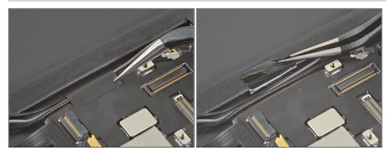
• Use a pair of tweezers to peel back the tape securing the Smart Connector cables to the rear case.
