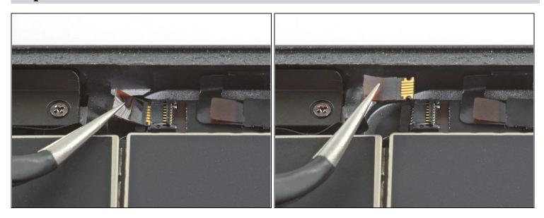
• Use a pair of tweezers to carefully pull the button control cable straight out of the ZIF connector.
