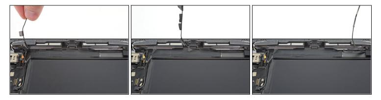
• Peel the left antenna cable away from the rear case, along the bottom edge of the iPad.
