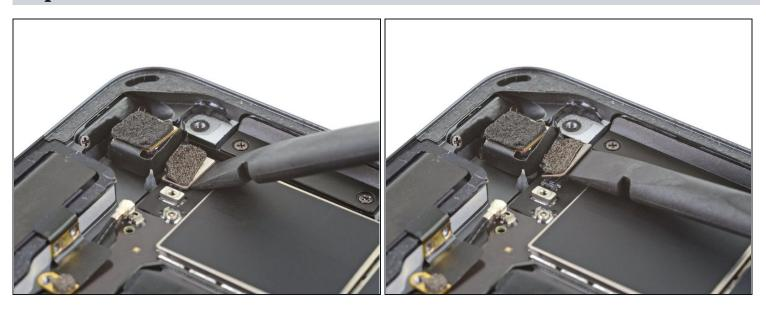
• Use the flat end of a spudger to disconnect the rear camera by lifting straight up on the press connector.
