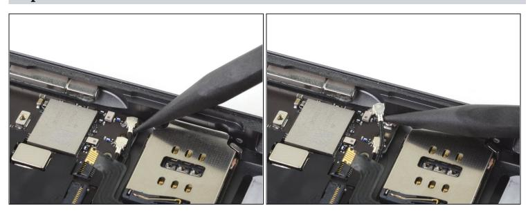
• Insert the pointed end of a spudger under the right antenna cable and lift straight up to disconnect it.
