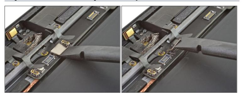
• Use the flat end of a spudger to disconnect the microphone assembly by lifting straight up on the press connector.
