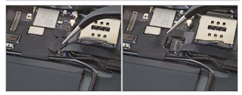
• Use a pair of tweezers to peel off the tape covering the home button cable ZIF connector.
