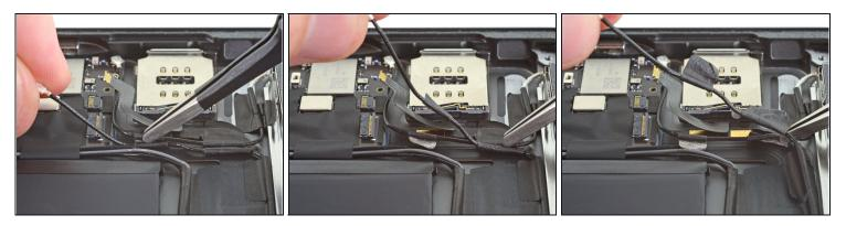
• Peel the left antenna cable up from the rear case.
