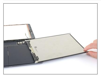
• Remove the LCD completely and rest it face down on a clean, soft, lint-free surface.
