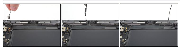
• Continue to peel the left antenna cable away from the rear case, along the bottom edge of the iPad.
