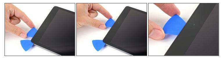
• Slide the opening pick along the top edge of the device, stopping just before you reach the front camera.
