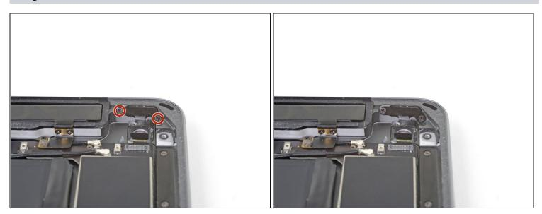
• Use a Phillips screwdriver to remove the two 2.3 mm-long screws securing the lock button bracket.
