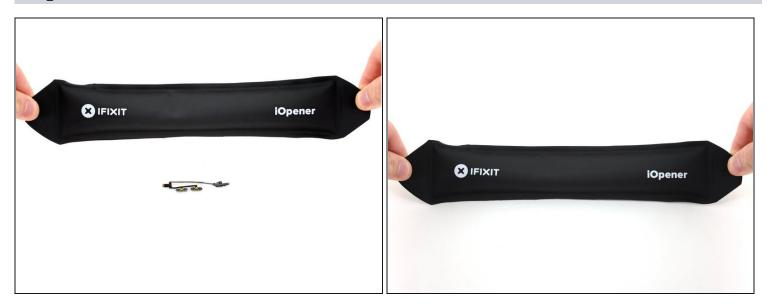
• <u>Heat an iOpener</u> and apply it to the button control cable for thirty seconds.
