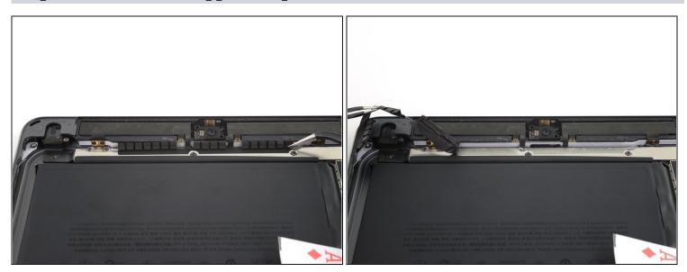
• Carefully peel the LCD buffer tape up off of the upper component bracket.
