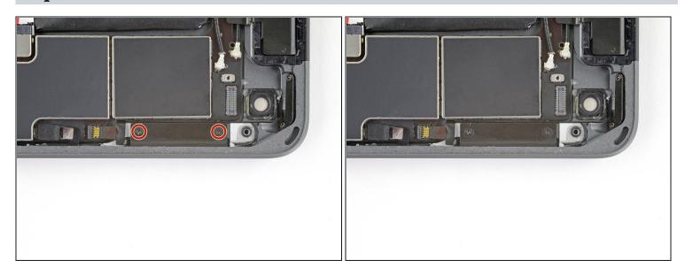
• Use a Phillips screwdriver to remove the two 2.3 mm-long screws securing the volume button bracket to the rear case.
