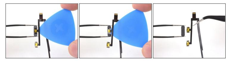
Repeat the same process to peel the volume control cable off of the lower volume button.
