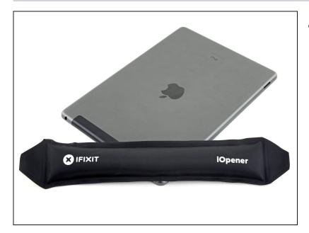
Heat an iOpener and apply it to the rear camera for thirty seconds.
