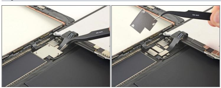
• Remove the display cable bracket.
