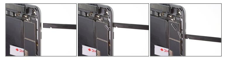
• Use the flat end of a spudger to push the volume buttons out of their slots in the rear case.
