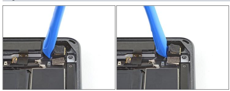
Use an opening tool to pry the rear camera out of the rear case.
