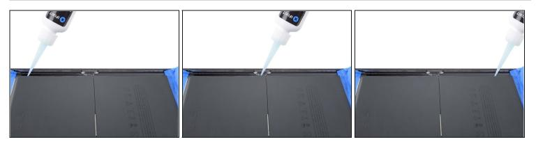
Apply a few drops of adhesive remover or high-concentration isopropyl alcohol along the left edge of the battery.
