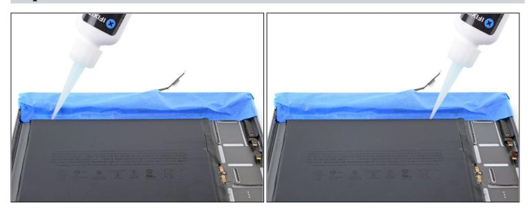
Apply a few drops of adhesive remover or high-concentration isopropyl alcohol along the upper edge of the battery.
