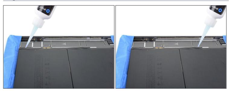
• Apply a few drops of adhesive remover or high-concentration isopropyl alcohol along the right edge of the battery.
