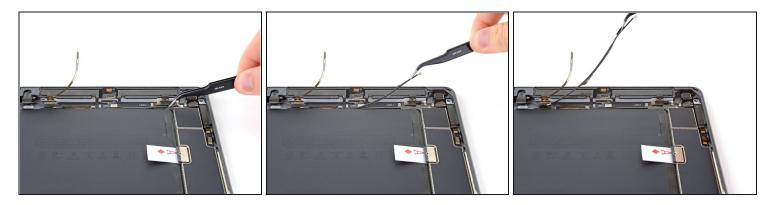
• Peel the left cellular antenna coaxial cable away from the rear case.
