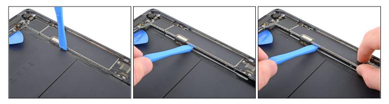
• Insert an opening tool near the middle of the logic board and pry up until you can grip it with your fingers.
