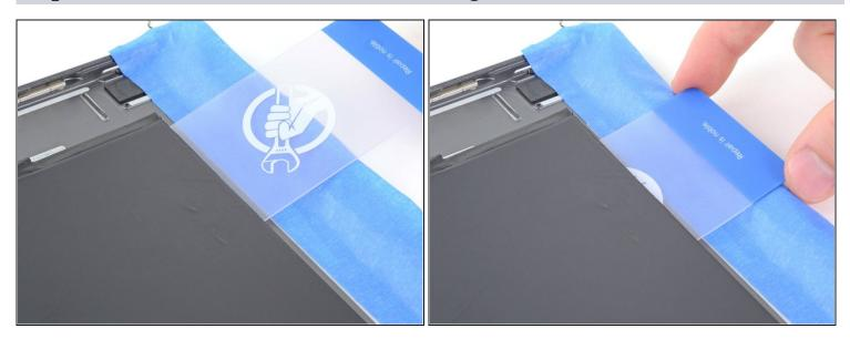
Remove the plastic card below the battery connector and insert it under the bottom edge of the battery.
