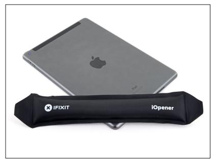
Heat an iOpener and apply it to the bottom left corner of the rear case to soften the SIM card reader's adhesive for thirty seconds.
