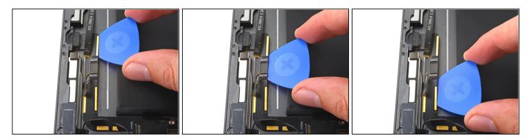
• Insert an opening pick under the charging port cable near the charging port and slide it towards the logic board to cut the adhesive.
