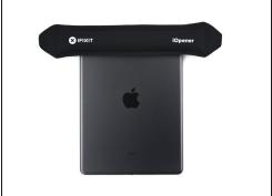
Heat an iOpener and apply it to the bottom, top, and logic board side of the iPad for thirty seconds in each location.
