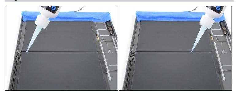
Apply a few drops of adhesive remover or high-concentration isopropyl alcohol between the two battery cells.
