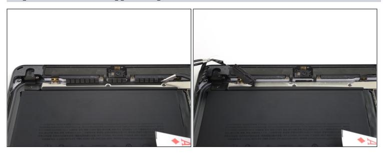
• Carefully peel the LCD buffer tape up off of the upper component bracket.
