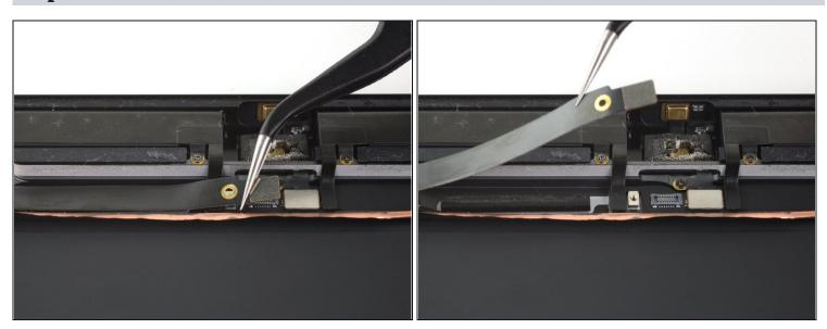
• Use a pair of tweezers to peel the headphone jack up from the logic board and fold the cable out of the way.
