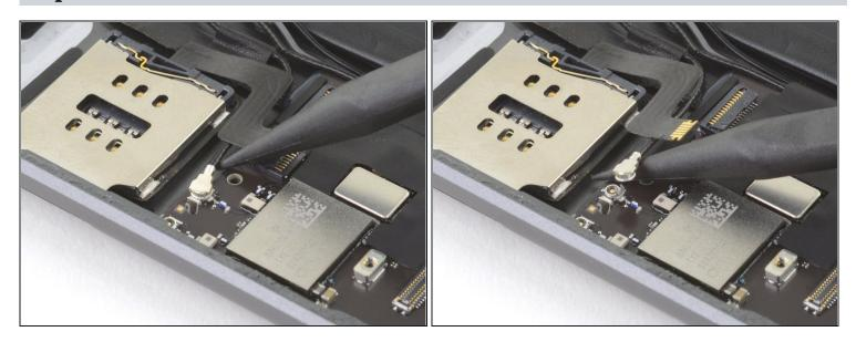
• Insert the pointed end of a spudger under the left antenna cable and lift straight up to disconnect it.
