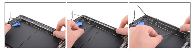
• Use a halberd spudger or an opening pick to slice any remaining adhesive securing the logic board to the rear case.
