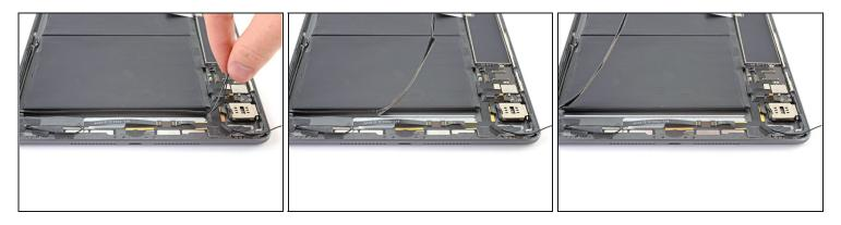
• Peel the Smart Connector cables away from the rear case.
