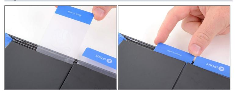
• When you reach the center edge, insert the plastic card as far as you can to cut the central adhesive strip.
