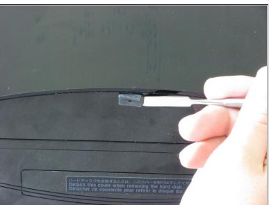
Remove the rubber screw cover near the hard drive cover with a spudger.
