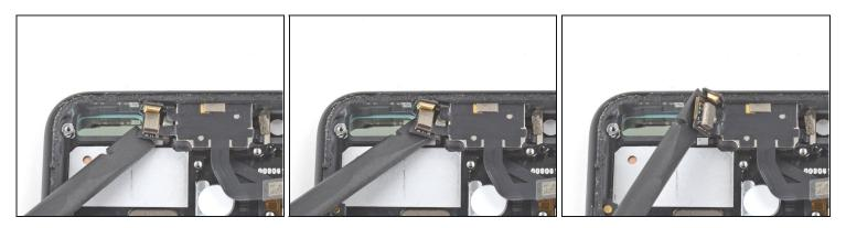
• Use the flat end of a spudger to slice through the adhesive securing the left side of the top module to the body of the frame.
