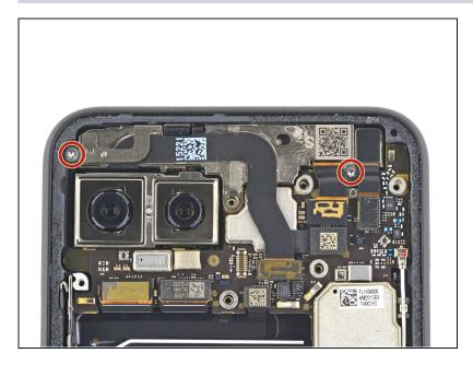
Use a T3 Torx driver to remove the two 2.4 mm screws securing the front camera and sensor assembly.
