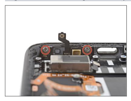
Use a T3 Torx driver to remove the two 3.3 mm shouldered screws securing the bottom microphone assembly to the frame's lower edge.
