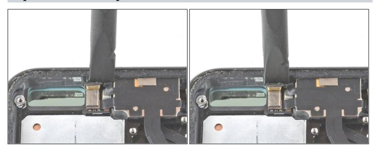
Use the flat end of a spudger to slice through the adhesive securing the top module to the top of the frame.
