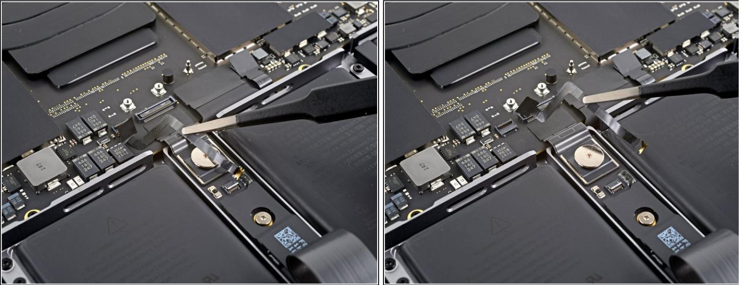
**i** The battery board data cable is lightly adhered to the device.
