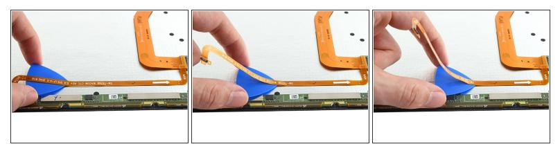
Slice with an opening pick along the bottom of the fingerprint sensor's cable to separate it from the screen.
