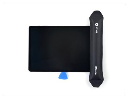
Apply a <u>heated iOpener</u> to the right edge of the device for two minutes to loosen the adhesive underneath.
