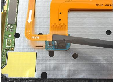
Use the flat end of a spudger to pry up and disconnect the fingerprint scanner cable's press connector from the screen.
