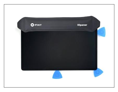
Apply a <u>heated iOpener</u> to the top edge of the device for two minutes to loosen the adhesive underneath.
