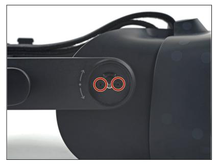
• Use a T6 Torx screwdriver to remove the two 6.6 mm screws underneath the eye relief knob.
