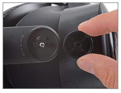
During reassembly, ensure the eye relief knob is aligned with the shaft before pressing it on.
