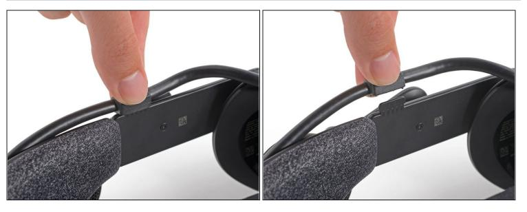
• Use your fingers to pull the tether cable straight up off of the head strap cable guide.
