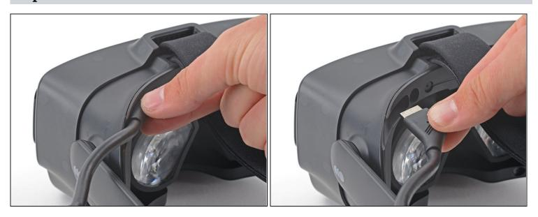
• Pull the tether cable straight back out of the headset.
