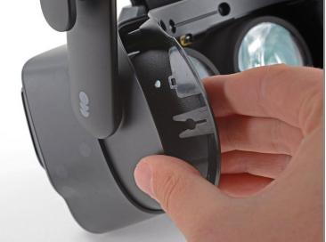
$\triangle$  Do not try and pry the face gasket bezel off, or you will damage the headset.
