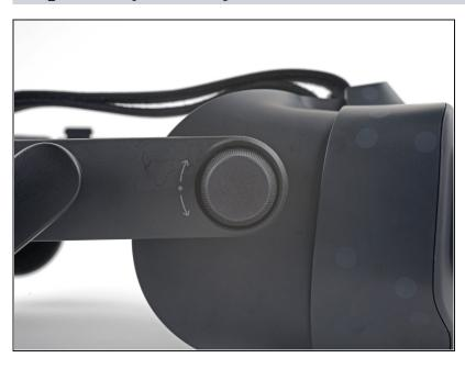
• Twist the eye tube relief knob clockwise to fully extend it.
