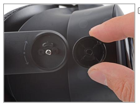
During reassembly, ensure the eye relief knob is aligned with the shaft before pressing it on.
