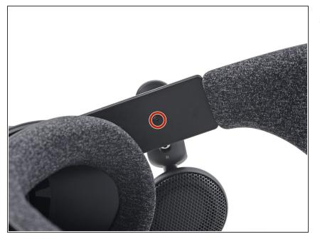
Use a T6 Torx screwdriver to remove the 8.1 mm screw securing the right speaker to the head strap.
