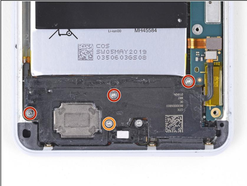
**i** If you have already removed the motherboard, the top right loudspeaker screw will already be removed.
