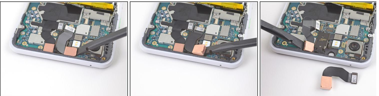
**i** The cameras are lightly adhered in place.
