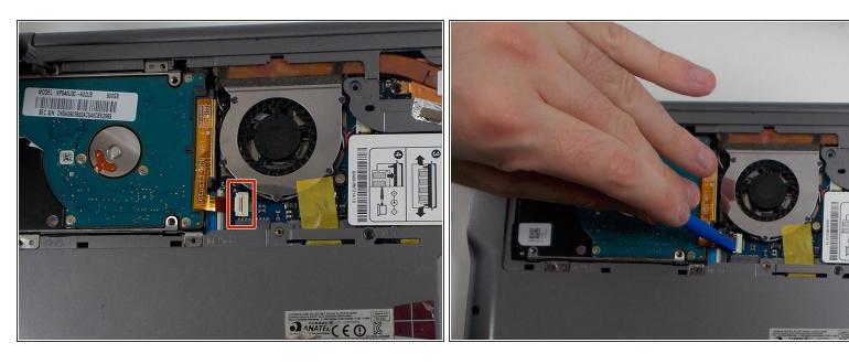
• Using the plastic opening tool, push the hard drive connector clip upwards in order to release the cable.
