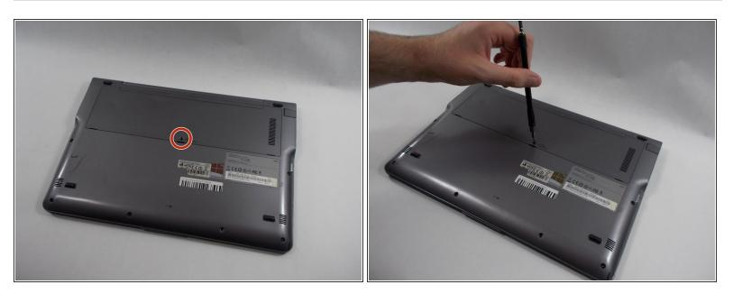
Remove the 1x 4mm Phillips #00 screw labeled "HDD Memory".
