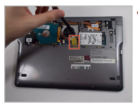
Peel the yellow tape up so it no longer blocks the fan's wires and screw.
