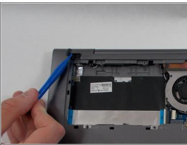
• Using the opening tool, remove the two rubber pads just above the hard drive cover.
