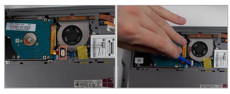
• Using the plastic opening tool, push the hard drive connector clip upwards in order to release the cable.
