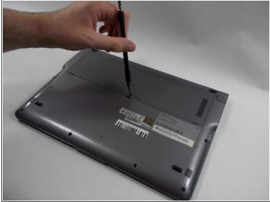
• Remove one 4 mm Phillips #00 screw labeled "HDD Memory".
