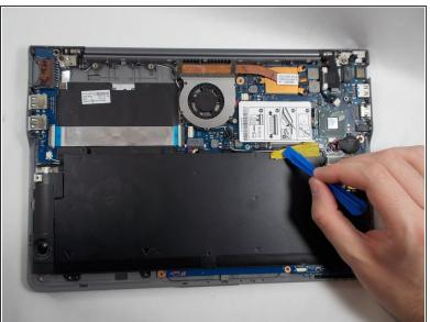
Using your hands or the plastic opening tool, gently remove the tape holding the wires in place.
