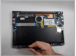
• Remove the 4x 4mm Phillips #00 screws securing the battery to the chassis.
