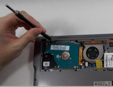
Remove the four 6 mm Phillips #00 screws attaching the hard drive to the case.
