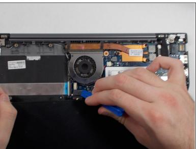
• Using the plastic opening tool, gently pull the battery connector towards the battery to disconnect it.
