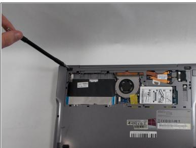
Remove the 2x 4mm Phillips #00 screws formerly concealed by the pads.
