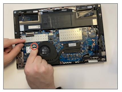
Disconnect the display panel cable from it's connector on the motherboard.
