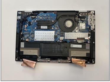
Peel back both sides of the copper foil tape connected to the battery.
