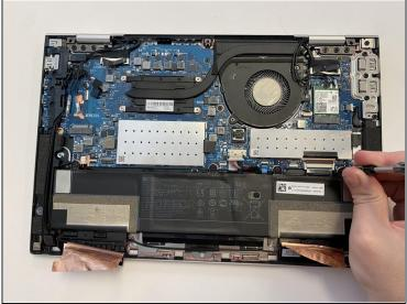
Use a JIS #1 screwdriver to remove the four 4 mm screws that secure the battery.
