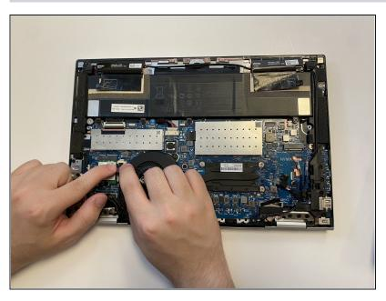
Remove the display panel and the wireless antenna cables from the routing channels. Then, remove the retention tape from the system fan.
