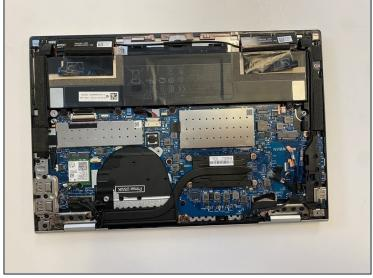
Once all of the connectors and screws that secure the fan in place have been removed successfully, you can safely remove the system fan from the motherboard.
