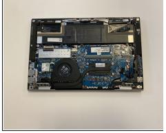
Gently lift the larger, rectangular metal shielding off. This shielding covers the RAM.
