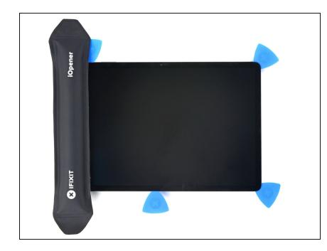
Apply a <u>heated iOpener</u> to the left edge of the device to loosen the adhesive underneath.
