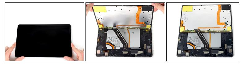
$\triangle$  Don't try to remove the screen all the way yet; it's still connected to the frame by a flex cable.
