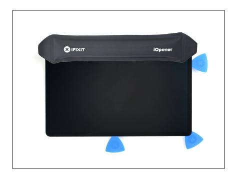
• Apply a <u>heated iOpener</u> to the top edge of the device to loosen the adhesive underneath.
