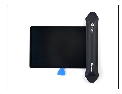
Apply a <u>heated iOpener</u> to the right edge of the device to loosen the adhesive underneath.
