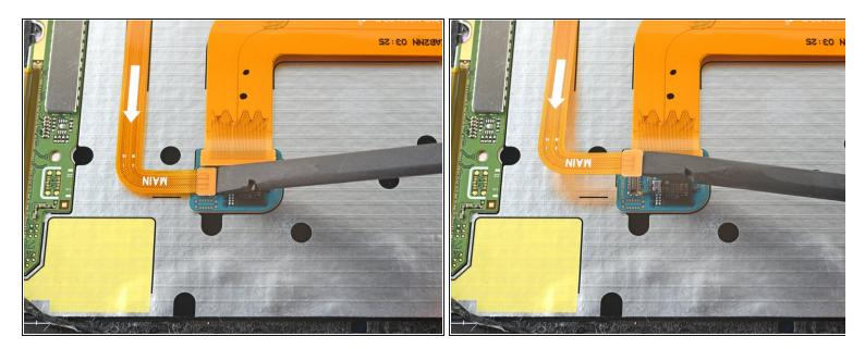
• Use the flat end of a spudger to pry up and disconnect the fingerprint scanner cable's press connector.
