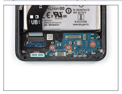
Use a Phillips screwdriver to remove the three 3.4 mm-long screws securing the charging board.
