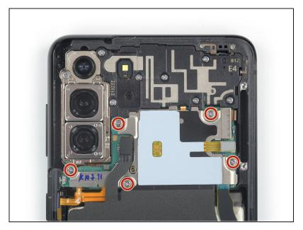
Use a Phillips screwdriver to remove the five 3.9 mm-long screws securing the NFC antenna and charging coil assembly.
