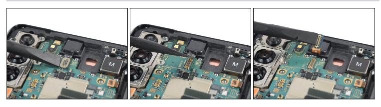
Use a spudger to disconnect the front facing camera cable by prying the connector straight up from its socket.
