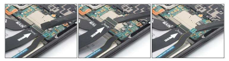
• Use a spudger to disconnect the main and interconnect flex cables from the motherboard by prying their upper connectors straight up from their sockets.
