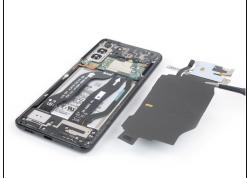
• Use a pair of <u>tweezers</u> or your fingers to carefully remove the NFC antenna and charging coil assembly.
