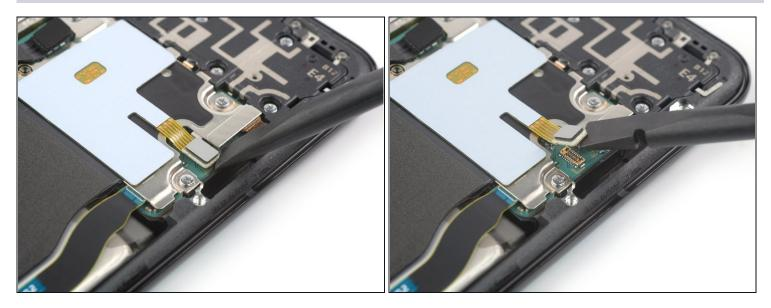
• Use a spudger to disconnect the NFC antenna by prying the connector straight up from its socket.
