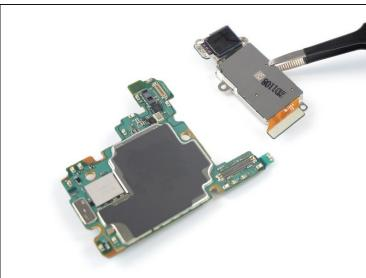
• Use a pair of <u>tweezers</u> or your fingers to carefully separate the camera assembly from the motherboard.
