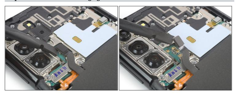
Use a spudger to disconnect the charging coil by prying the connector straight up from its socket.
