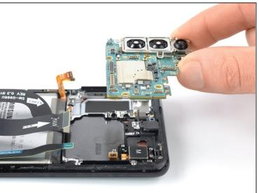
• Carefully remove the motherboard assembly including the rear cameras.
