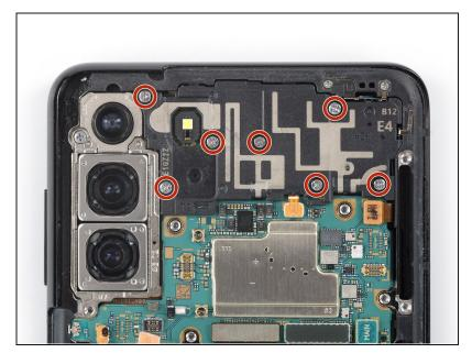
Use a Phillips screwdriver to remove the seven 3.9 mm-long screws securing the earpiece speaker assembly.
