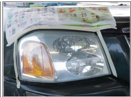
• Use 70% isopropyl alcohol and paper towels to remove any residue on the headlights.
