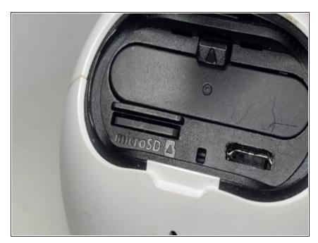
Eject the SD by pushing with your fingernail or flathead screwdriver.
