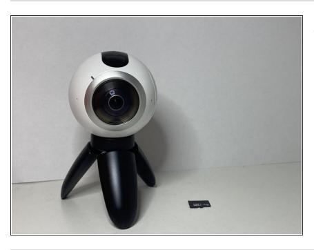
After removing the SD Card, insert a new one and finish the guide!!
