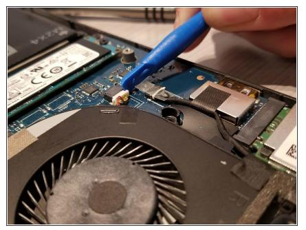
• Use the Small Plastic Spudger to carefully disconnect the white connector from the black port.
