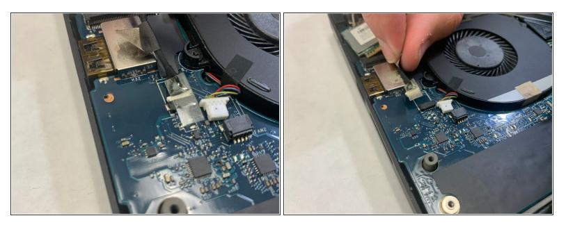
• This connector in the top left might be taped in two places. Simply pull up to loosen the tape, and use the plastic edges of the connector to pull it out. Have some tape on hand for reassembly, as the tape might have lost its adhesive backing.
