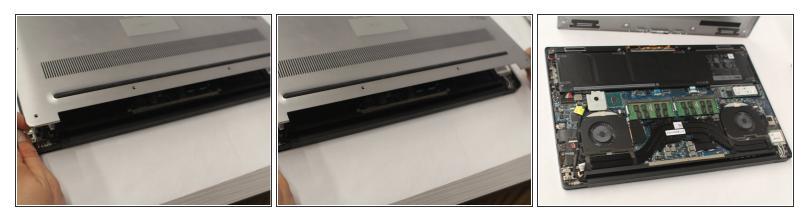
Carefully lift the 2 corners of the back panel close to the hinge upwards, to release the whole panel.
