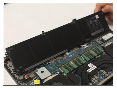
• Gently lift up on the backside of the battery.
