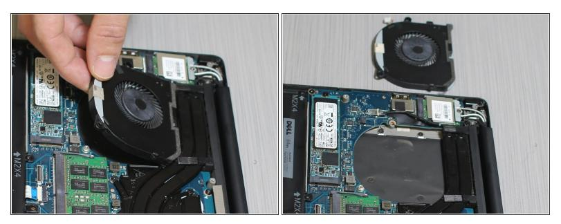
• With the screws removed, lift up on the fan and remove it from the laptop.
