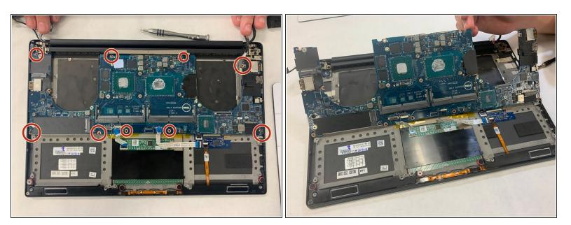
With all mounted components removed, unscrew the motherboard Phillips-head screws.
