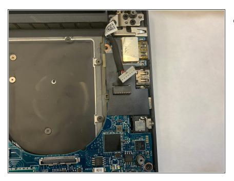
Pull this Monitor connector out by its plastic edges
