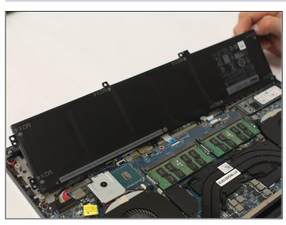
• Gently lift up on the backside of the battery.
