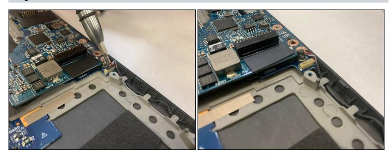
• Pull up on the plastic edges to remove the indicated connector at the bottom right of the motherboard.
