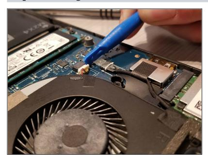
Use the Small Plastic Spudger to carefully disconnect the white connector from the black port.
