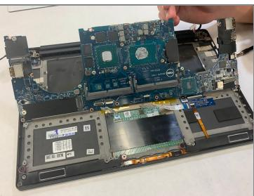
With all mounted components removed, unscrew the motherboard Phillips-head screws.
