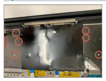
Remove 6 exposed #00 Phillips screws from the center of the keyboard.
