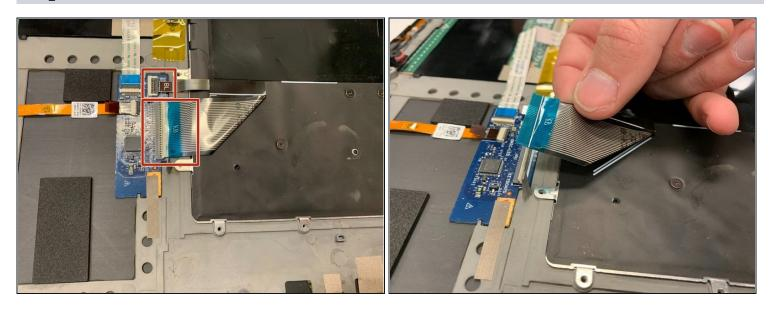
• Unplug the keyboard from the laptop by flipping up the small ZIF tabs and pulling the ribbon cables straight out.
