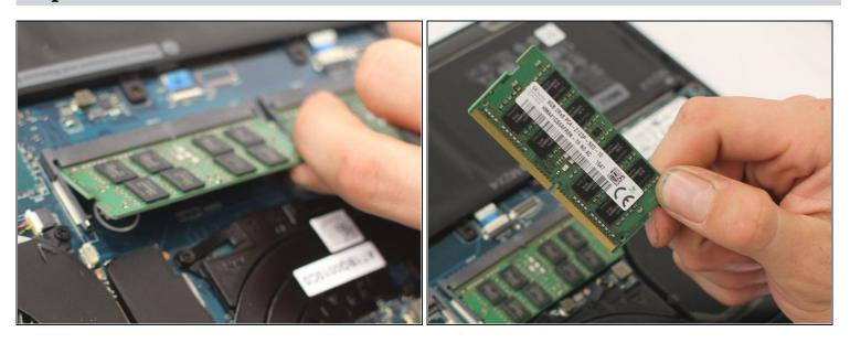
• Firmly grasp the RAM stick from the flipped up edge and gently pull out, to release the RAM stick.
