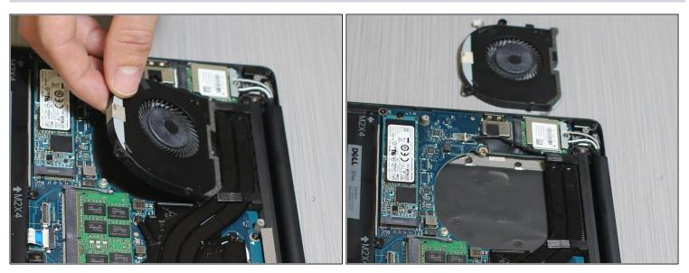
• With the screws removed, lift up on the fan and remove it from the laptop.
