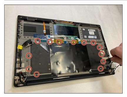
• Remove the 14 #00 Phillips screws from the perimeter of the keyboard.
