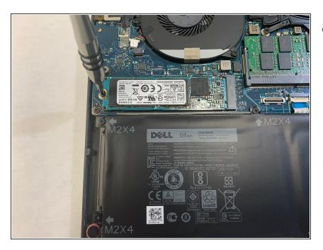
Use a Phillips #00 screwdriver to remove the SSD screw.
