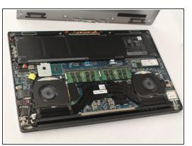
Carefully lift the 2 corners of the back panel close to the hinge upwards, to release the whole panel.
