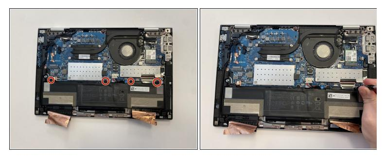
• Use a JIS #1 screwdriver to remove the four 4 mm screws that secure the battery.
