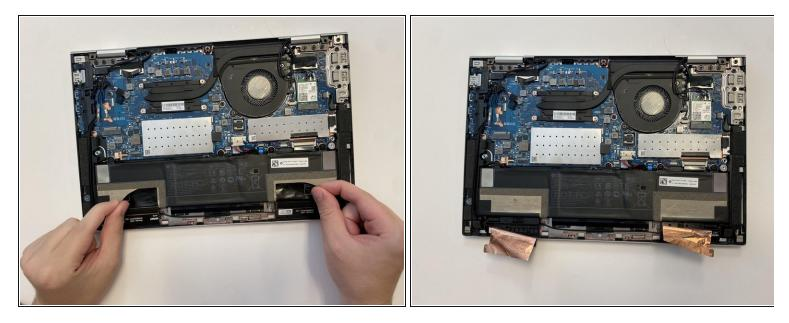
• Peel back both sides of the copper foil tape connected to the battery.
