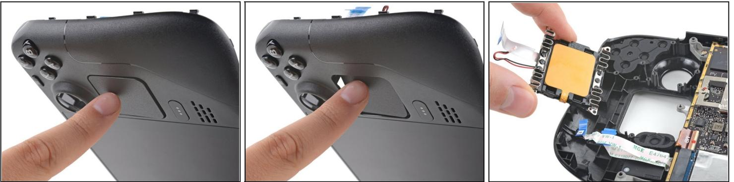
⚠ The touchpad's springs are very delicate and are precisely positioned. If bent, the touchpad may rattle or not work as intended.
