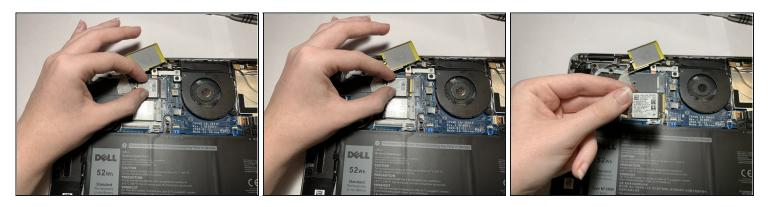
• Grip the SSD and pull directly backward until the SSD releases from its port.
