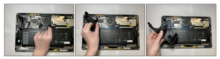
• Carefully peel back and remove the black tape around the top left corner of the motherboard.
