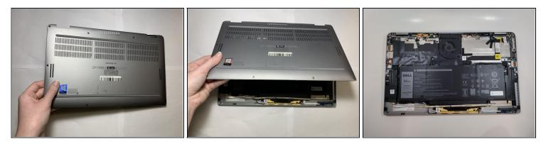
• Carefully lift off the back panel.
